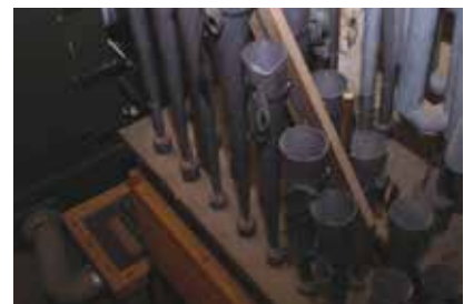
Reed pipes damaged by improper tuning: the tops have been squashed, also affecting the tone.
